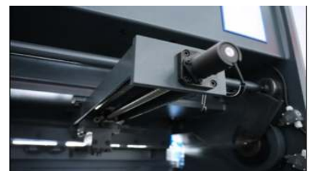
Backgauge With Double Lm Guides & Ball Screw
