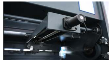
Backgauge With Double Lm Guides & Ball Screw
