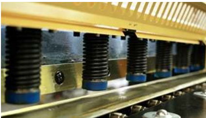
High Tensile Strength Hold Downs
