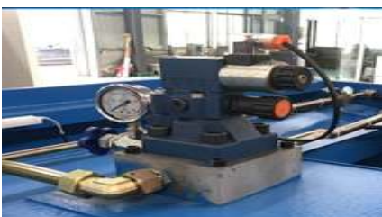
Germany Bosch Rexroth Hydraulic System
