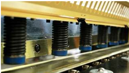
High Tensile Strength Hold Downs
