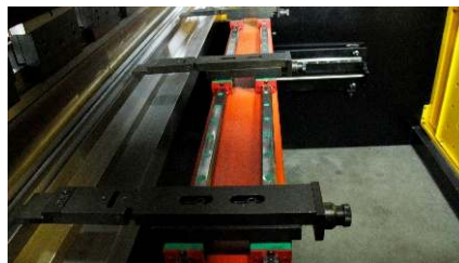
Stop Finger With Double LM Guide
