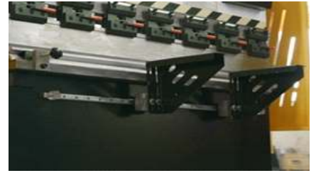
Front Material Support With LM Guide
