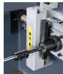
R Axis - With Rack And Pinion And LM Guide
