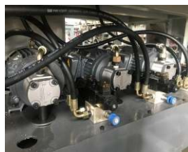
Separate Ele. Motor & Hydraulic Pump for each working station.
