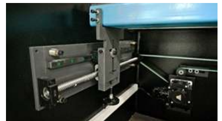
Backgauge With LM Guides & Ball Screw
