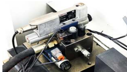
Proportional Valve - Rexroth (Y1 & Y2)
